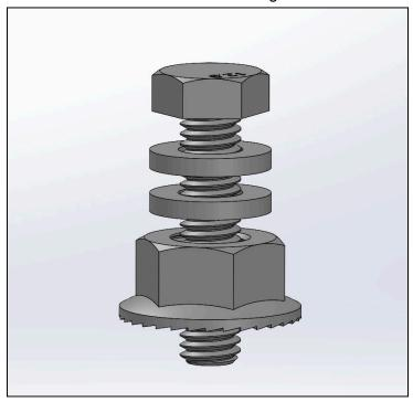
Once done, screw the nut up just enough such that the rivet can be threaded to be flush with the end of the bolt
