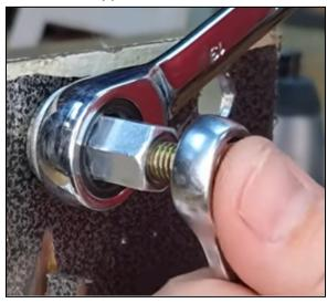
Once your hardware is in this position, crank the 13mm ratchet wrench around the nut (clockwise) while holding the hex bolt in place with the 10mm socket wrench. Do this until the rivnut compresses into the hole and the fixture becomes almost impossible to turn.
